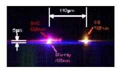
Sony Corporation has developed a single **3-wavelength recording/playback optical head**, capable of recording and playing-back 3 formats, Blu-ray Disc (BD), in addition to DVD, CD, which is a high-density optical disc system capable of recording/playing back high definition contents.
