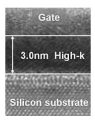
After several years of effort, the Intel technology team has made a major breakthrough that solves the chip power problem. Intel has identified a new material known as "high-K" to replace SiO2 as the gate dielectric, in addition to new metals to replace the polysilicon gate electrode of NMOS and PMOS transistors.
