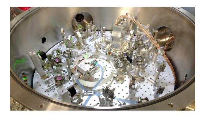
A new squeezed vacuum source could make gravitational wave detectors sensitive enough to study neutron stars. Credit: Eric Oelker, Massachusetts Institute of Technology
