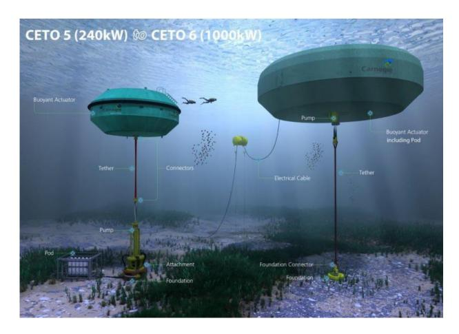
Artist' concept of a series of the Carnegie Wave Energy's tidal system, where buoys anchored to the sea floor and use swells to move a series of pumps. Credit: Carnegie Wave Energy
