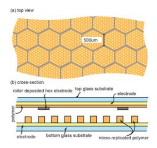
Top view and side-view diagrams of the device construction.
