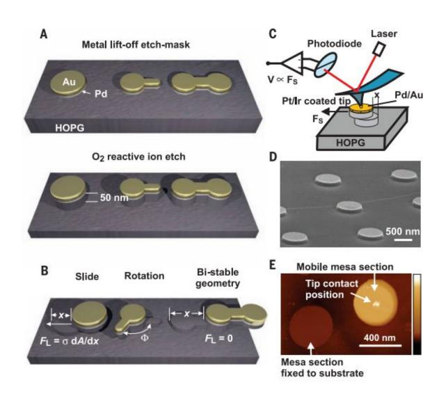
Experimental procedures. (A) Metal masks consisting of Pd (10 nm) and Au (15 nm) are fabricated on the freshly cleaved surface of a HOPG sample by electron beam lithography and liftoff techniques. The mesa structures emerge during a
