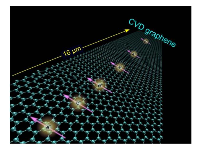
In graphene, electrons keep their magnetization, their spin (the pink arrows in the picture) much longer than they do in ordinary conductors such as copper and aluminum. This characteristic of graphene may enable spintronics to become a complement to traditional electronics, which only utilizes one of the electron's degrees of freedom, namely their charge. Credit: M Venkata Kamalakar et al, *Nature Communications*
