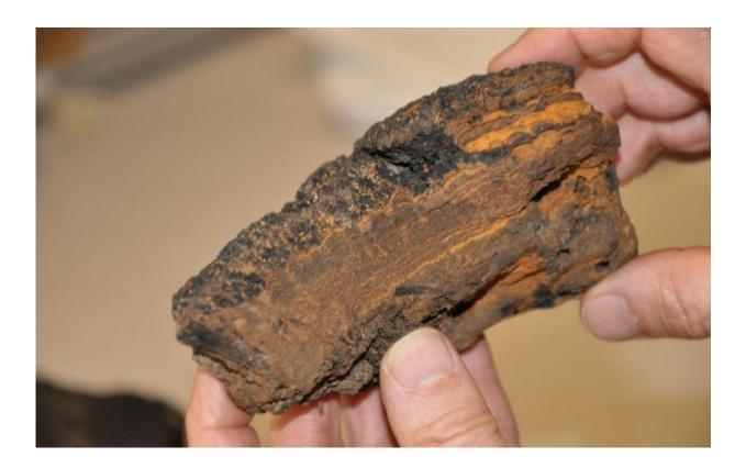
Ferromanganese crusts with typical band structure. Credit: Source: Buczkowski, USGS.
