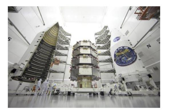
In preparation for launch, four stacked observatories are loaded into the fairing of the Magnetospheric Multiscale spacecraft launch vehicle. Southwest Research Institute leads the science investigation for MMS, a NASA mission to study magnetic reconnection up close for the first time. Credit: NASA/Ben Smegelsky
