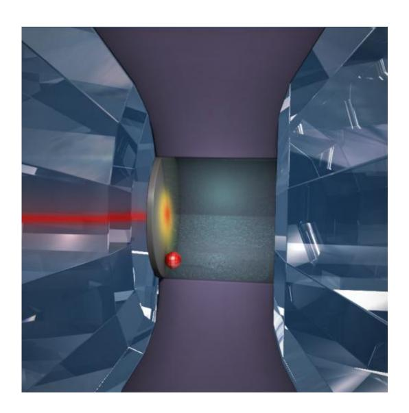
Artist's rendition of the high pressure thermal conductance experiment in a diamond anvil cell. The flat tips of the diamond anvils are less than half a millimeter in diameter, and the metal film (gray), ruby sphere (red), and pressure medium (blue fluid) are sealed between the diamonds by a metal gasket (solid
