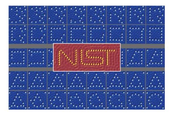
Automated assembly of individual cobalt atoms on an atomically flat copper surface into simple geometric shapes, a square, a triangle, and a circle. From left to right, each figure shows the configuration after each atom move. Image size 15 nm  $\times$  15 nm. Center: Perfect assembly of the NIST logo after four steps of automated assembly. Image size 40 nm  $\times$  17 nm. All images are shown in colored 3D top view with light shadowing with a height range of  $\approx$ 100 pm.
