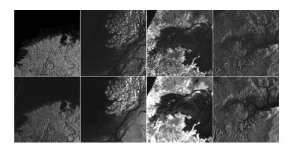
This montage of Cassini Synthetic Aperture Radar (SAR) images of the surface of Titan shows four examples of how a newly developed technique for handling noise results in clearer, easier to interpret views. The top row of images was
