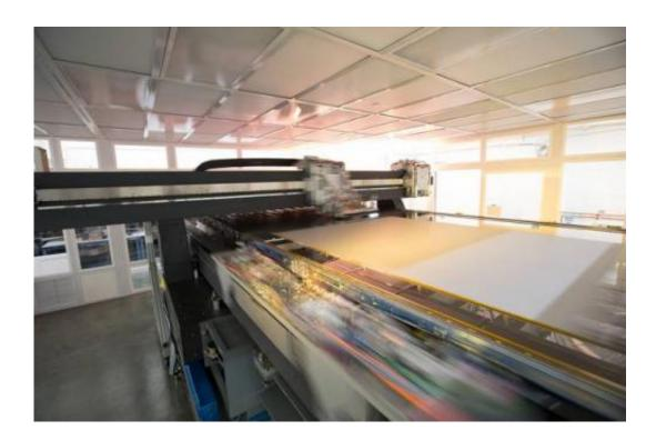
Kateeva's YIELDjet system (pictured here) is a massive version of an inkjet printer. Large glass or plastic substrate sheets are placed on a long, wide platform. A head with custom nozzles moves back and forth, across the substrate, coating it with OLED and other materials. Credit: Kateeva
