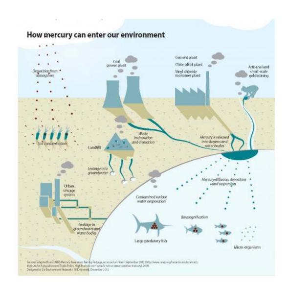
This graphic shows how mercury can enter the environment. Credit: UNEP Chemicals Branch, DTIE - Switzerland
