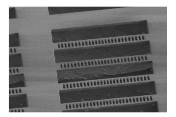
The researchers' device is a ladderlike structure etched into diamond. The gaps between the ladder's "rungs" act like a mirror, temporarily trapping light particles emitted at the ladder's center.
