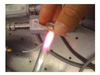
A microscopic plasma formed by a microwave circuit board creates a large plume of plasma inside a glass tube. Credit: Jeff Hopwood
