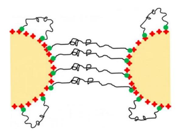
DNA linkers serve as bridges between colloidal beads in a new experiment by Rice University scientists to study the physics of "bead-spring" polymer chains. They found the chains can be tuned for varying degrees of stiffness or flexibility. Credit: Biswal Lab/Rice University
