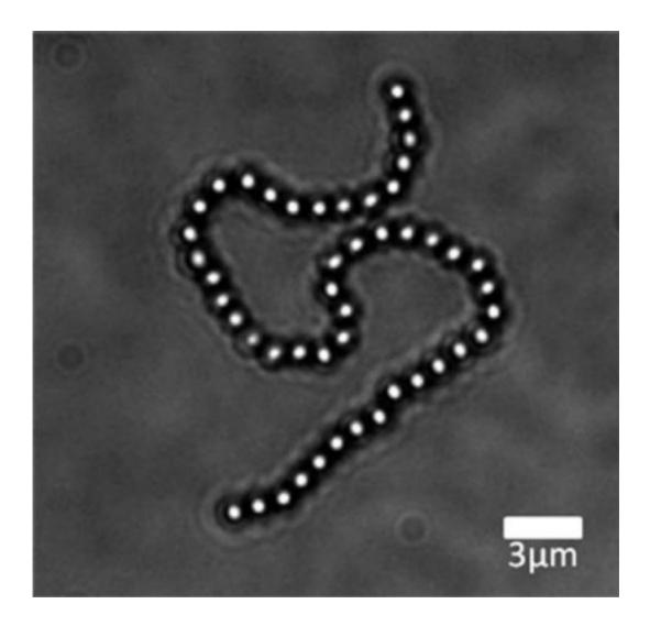
Chains of iron-rich polystyrene beads linked by nanoscale strands of DNA were created at Rice University to study the properties of "bead-spring" polymer chains. Credit: Biswal Lab/Rice University
