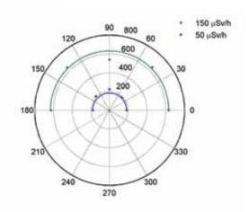
Figure 3: The angular response of the Samsung Galaxy S2 smartphone at two different dose rates, 50  $\mu$ Sv/h and 150  $\mu$ Sv/h.The dots represent the number of counts recorded by the phone at different orientation angles.
