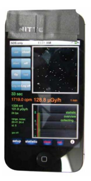
Figure 1: This shows the display the iPhone with the app running and a 137Cs source placed behind the phone. The top right panel shows the response of the
