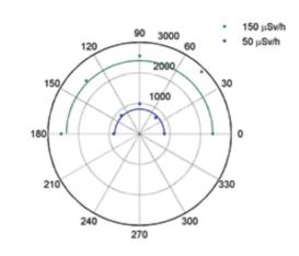
Figure 4: The angular response of the iPhone 4S smartphone at two different dose rates, 50  $\mu$ Sv/h and 150  $\mu$ Sv/h. The dots represent the number of counts recorded by the phone at different orientation angles.
