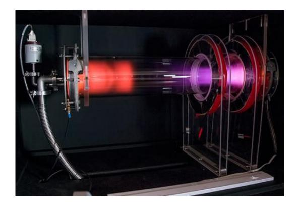
Above, a plasma glows in the RGDX. The experiment involves a glass tube connected to a vacuum pump, encircled by two electromagnetic coils and linked to electrodes at either end of the device. Users can use the controls to change the pressure in the tube, the voltage between the electrodes and the strength of the magnetic field to create the plasma and to make it glow.
