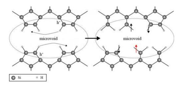
In the initial state (left), the voids' internal surfaces are saturated with hydrogen atoms so that no defects are observed. Light-induced charge carriers (h+) destabilize atomic bonds. The breaking of atomic bonds causes defects (indicated by the vertical arrows on the right hand side), which translates to reduced solar cell efficiency. Credit: HZB
