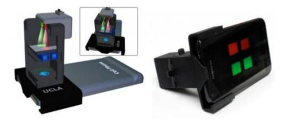
A smartphone attachment developed at UCLA Engineering tests water for mercury contamination. The new platform could significantly reduce the time and cost of the testing.
