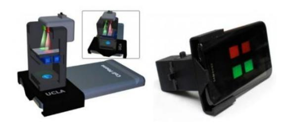
A smartphone attachment developed at UCLA Engineering tests water for mercury contamination. The new platform could significantly reduce the time and cost of the testing.
