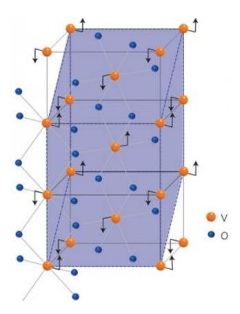
A schematic of the crystal structures in VO2, showing the motion of the vanadium (black arrows) with respect to the oxygen ions across the metal-insulator transition. VO2 acts like an insulator at low temperatures but like a metal at near room temperature.
