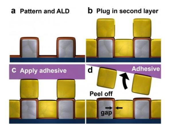
In a breakthrough study to improve the manufacturing of optical and electronic devices, University of Minnesota researchers introduced a new patterning technology, atomic layer lithography, based on a layering technique at the atomic level. A layer of metal fills the nano-patterns over an entire wafer and simple Scotch Magic tape was used to remove the excess metal on the surface and expose the atomic scale nano-gaps.
