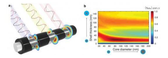
The core-shell hybrid nanowire consists of a metal core wrapped with semiconductor thin films. Three different resonances excited at different wavelengths are shown. (b) The fraction of absorbed above-band gap photons in the silicon shell for a wide variety of configurations. Credit: Mann and Garnett. ©2013 American Chemical Society
