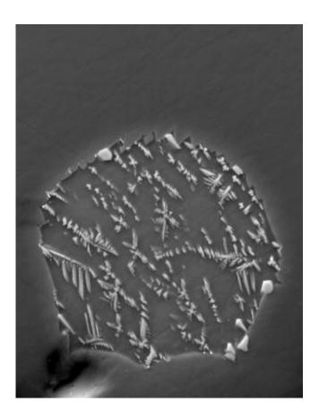
Backscatter electron image of a lunar melt inclusion from Apollo 17 sample 74220, enclosed within an olivine crystal. The inclusion is  $30 \ \mu m$  in diameter. Skeletal crystals within the melt inclusion are a fine mixture of olivine and ilmenite. Dark area in the lower-left is an ion microprobe sputter crater. Credit: John Armstrong, Geophysical Laboratory, Carnegie Institution of Washington
