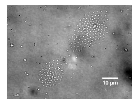
Here the technique, called rapid electrokinetic patterning, is used to arrange the bacteria into a speific pattern. The technique may be used as a tool for nanomanufacturing because it shows promise for the assembly of suspended particles, called colloids. The ability to construct objects with colloids makes it possible to create structures with particular mechanical and thermal characteristics to manufacture electronic devices and tiny mechanical parts. Credit: Purdue University
