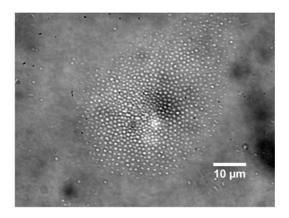
Researchers have demonstrated a new technology that combines a laser and electric fields to create tiny centrifuge-like whirlpools to separate particles and microbes by size, a potential lab-on-a-chip system for medicine and research. Here the technique is used to collect a bacterium called *Shewanella oneidensis*. Credit: Purdue University
