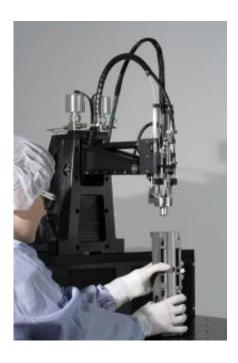
This cleaning tool removes even every fine dirt particles from areas inside components that are difficult to clean, for example boreholes and blind holes. Credit: Fraunhofer IPA
