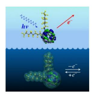
The figure depicts the processes of removing an electron from the negatively-charged radical anion of 1,7-C60(C8F17)2, in the gas-phase by low-temperature photoelectron spectroscopy and in solution by cyclic voltammetry. Image by Alexey A. Popov,
