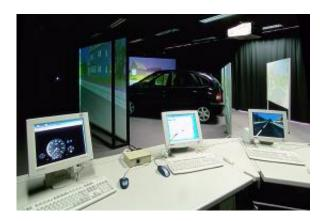
Driver fatigue is a common cause of road accidents. A new system warns drowsy drivers before it's too late. At the Vehicle Interaction Lab, researchers are studying in a virtual environment how best to design the electronic monitoring system by focusing on the human element.
