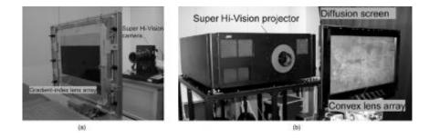
The experimental setup for (a) capturing video and (b) displaying video. Both steps involve a large array of convex lenses to generate a 3D effect. Image credit: Arai, et al. (c)2010 IEEE.
