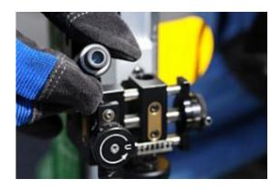
The MicroSight's wafer-thin optical element is only about a quarter-inch in diameter.
