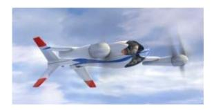
(PhysOrg.com) -- NASA engineers have designed an extremely quiet one-person electrically powered aircraft that can hover like a helicopter and fly like a plane. The "Puffin" launches from an upright position with the tail split into four legs that serve as stable landing/take-off gear.
