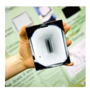
A blast from a heat gun has turned most of the black tile in this image white. The prototype tile, developed by recent MIT graduates, is designed to turn dark in cold weather and white in warm weather. Image: Patrick Gillooly
