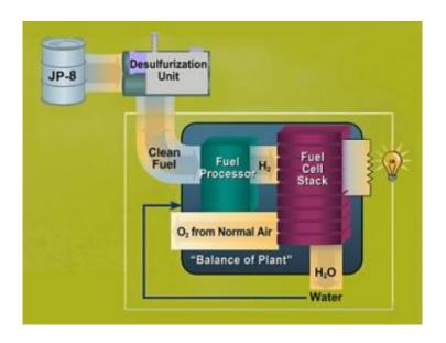
The process of converting JP-8 into hydrogen for use in the on-board fuel cell. Credit: Pacific Northwest National Laboratory
