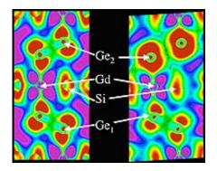
Spin density contour plots for Gd5Si2Ge2 show dramatic changes when Ge2 covalent bonds break at the magnetostructural transition responsible for the giant magnetocaloric effect in this material. (Calculations by Y. Lee and B. Harmon.)
